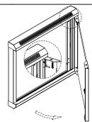
2 Use the included key to pull open the door (1) and remove it from the front frame (2) by pushing down on the latch.
