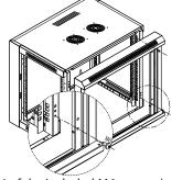
**6** Use 4 of the included M6 screws (use 6 for larger units) to attach the front frame (**2**) to the assembly.
