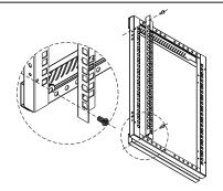
**3** Use the 4 included M5 screws to attach a mounting rail (**7**) to each side frame (**3**).
