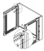
**4** Use 4 of the included M6 screws (use 6 for larger units) to attach each of the 2 side frames (**3**) to the back frame (**6**).
