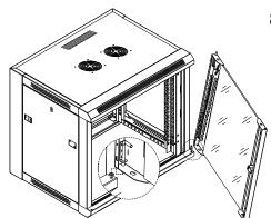
**8** Reverse Step 2 by inserting the lower door latch into the frame and then pushing down on the upper door latch to install the front door (1). Note: Once the unit is assembled, check that all corners are square to ensure that the door opens and closes properly.
